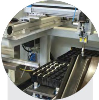
A pick&place system packs the tested and processed parts, e.g. in trays.
